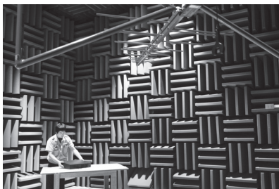
Acoustic radio wave anechoic chamber
